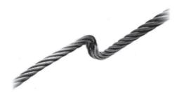
3. The result: Even if the wires do not appear badly damaged, the rope is still damaged and must be replaced.
