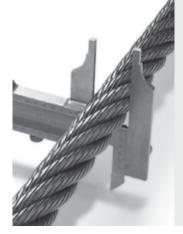
he actual diameter of a wire rope is the diameter of a circumscribed circle that will enclose all the strands. It's the largest cross-sectional measurement as shown here. You should make the measurement carefully with calipers. The illustrations at left show the correct and incorrect methods of measuring wire ropes with even numbers of outer strands.
