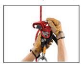
The descender has a safety gate on the moving side plate that allows the rope to be installed easily while the device remains connected to the harness.
