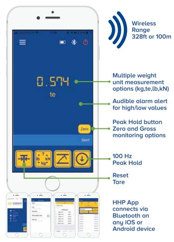
Designed to replace outdated mechanical products still in the field, this 14,300lb (6500kg) Dynamometer, the 'BlueLink', is the latest SP product to feature their proprietary Bluetooth wireless technology.
