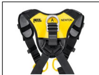
The metal dorsal attachment point allows attachment of a fall-arrest system, and the textile dorsal attachment point allows attachment of a self-retracting fall-arrest system.
