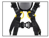
The FAST LT PLUS sternal buckle allows the harness to be quickly and easily fastened and unfastened without loss of adjustment, even with gloves. Lightweight and strong, the textile sternal attachment point allows attachment of a fall-arrest system.
